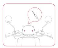
Align the windshield rubber part with the windshield holes and then install it.
