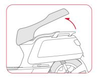
Open the saddle to take out the key box, windshield package (with rubber pads and standard parts), and installation tools.
